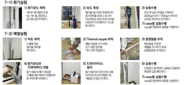
Fig. 3. The process of production of experiment and experiment setup
